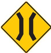
Narrow structure ahead — often a bridge
